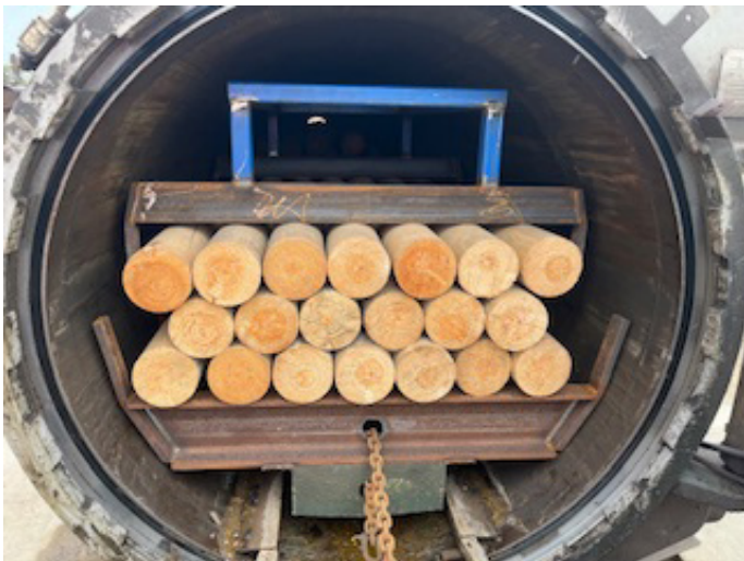
Treatment Plant Frame
